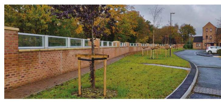
Specifically, IBS installed six floodgates, with the largest of these being a double-leaf mitred design at 10m wide and with one half containing a glass top section. In addition, IBS also installed approximately 340m of glass flood wall systems throughout the scheme, in various layouts and sections at typical heights of 600mm and 900mm.
